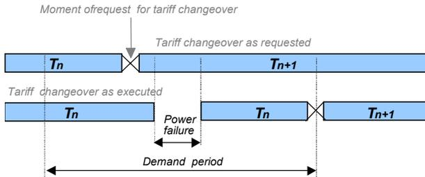
Fig. 40: Tariff changeover delay in case of a power shortage
