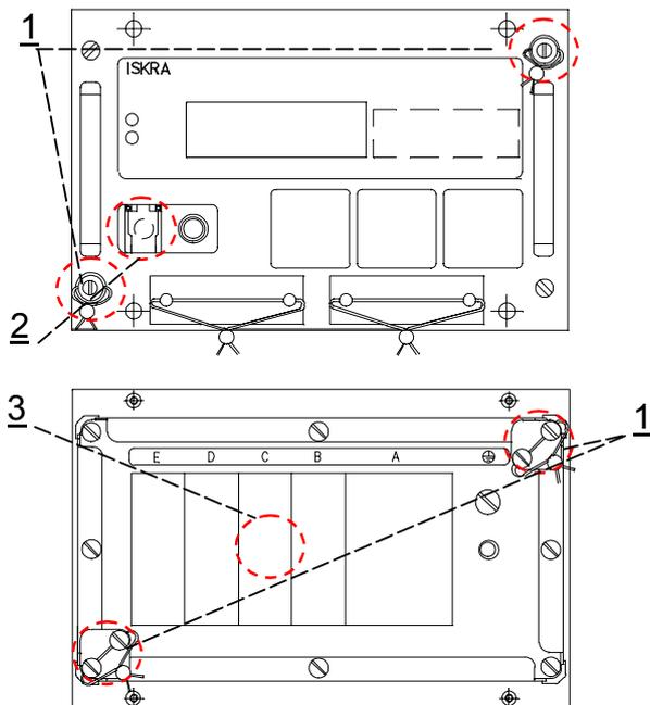
Fig. 41: Places of sealing: 1-meter cover, 2-reset button, 3- ESSAILEC connectors.
