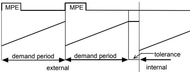
Fig. 35: Demand not measured in a tolerance time
