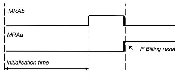
Fig. 28: MRa MRb outputs at restart and first billing reset
