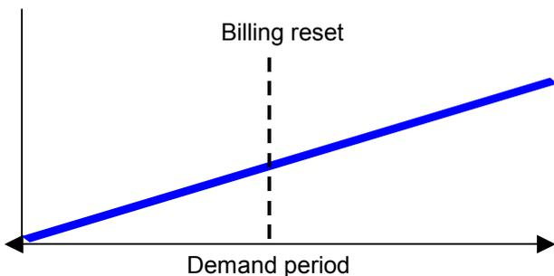
Fig. 37: Billing reset does not interrupt demand period
