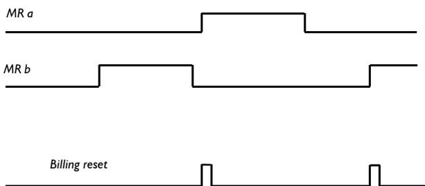
Fig. 42: MRa and MRb signals perform billing reset.
