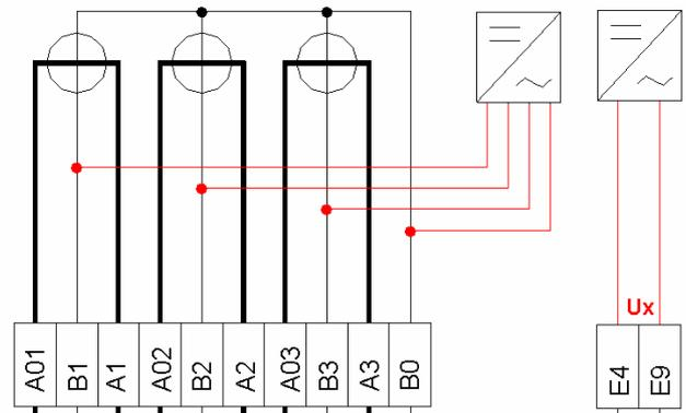
Fig. 31: Internal and external power supply
