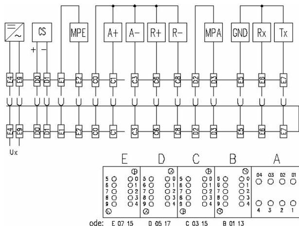
Fig. 5: ESSAILEC connector scheme
