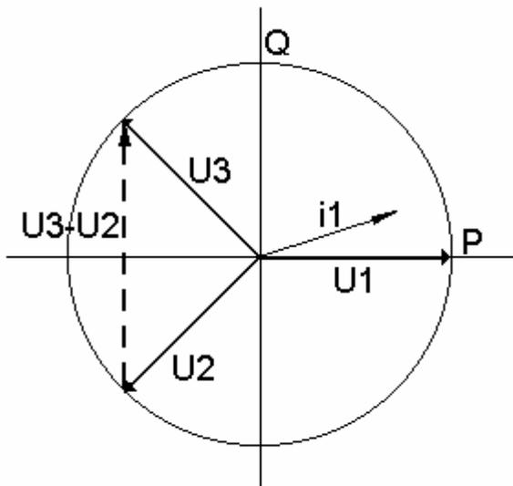
Fig. 13: Artificial connection voltage vector diagram
