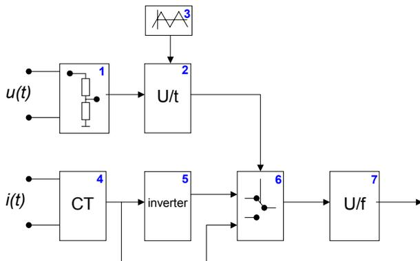
Fig. 7: TDM measuring system
