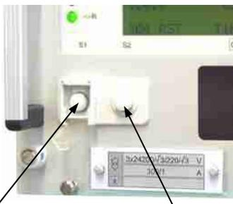
Reset pushbutton      Scroll pushbutton
