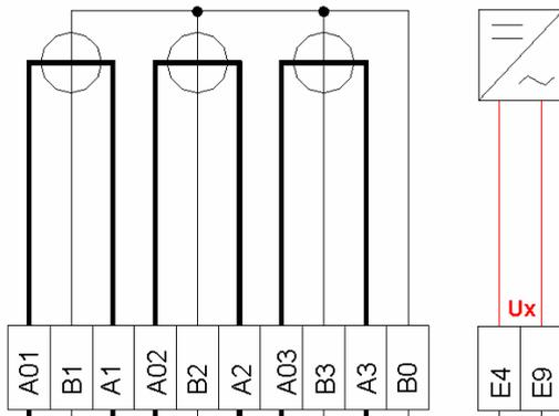
Fig. 30: External power supply  $U_x$
