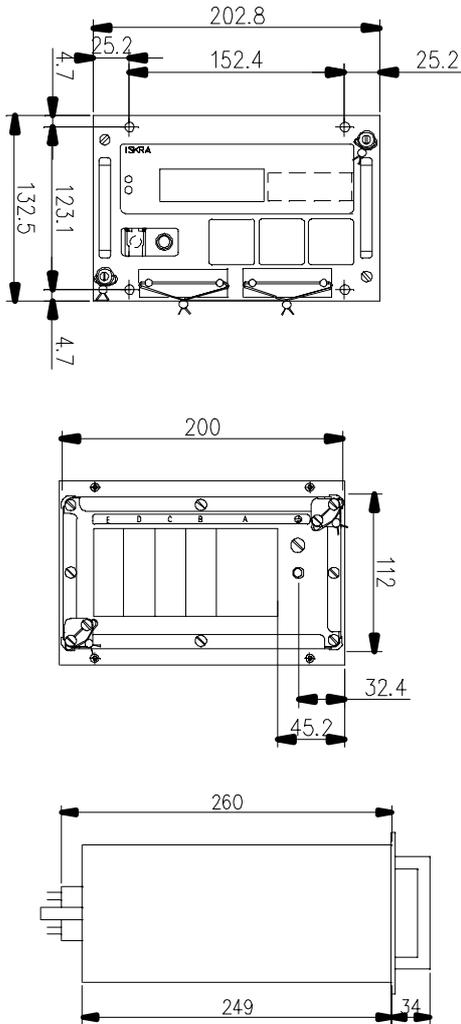
Fig. 3: Meter housing dimensions
